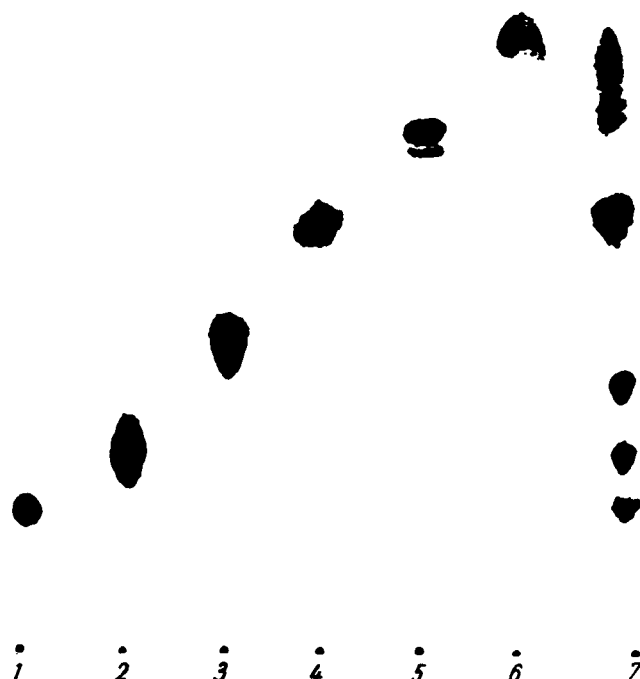
FIG. 16. Separation of phospholipids on Silica Gel. (219, 220). Solvent: chloroform-methanol-water, 65/25/4, v/v/v. Development time: 2 hours. Indicators: Rhodamin B and Dragendorff reagent. Amounts: 50-100 \gamma , each. 1) lysolecithin, 2) sphingomyelin, 3) lecithin, 4) cephalin, 5) cerebroside, 6) cardiolipid, 7) mixture.
